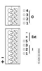
Wiring diagram digital 24 V DC communication for 1 solenoid valve and 3 outputs:
